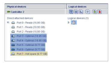
The Full Size Capacity View of the same RAID 5 logical drive shows that the two larger disk drives still have available space (free segments, indicated in light-blue) that is not part of a logical drive.
