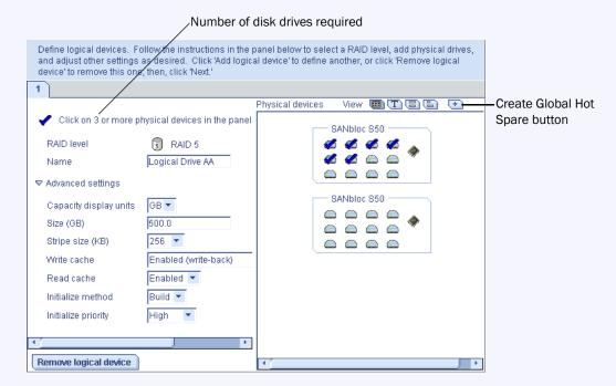
This figure illustrates disk drives installed in two enclosures.
